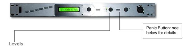
The level control is both a knob and a switch. Use it as a switch to select which level you want to adjust, and use it as a knob to adjust the level, which will appear in the LCD Display.
